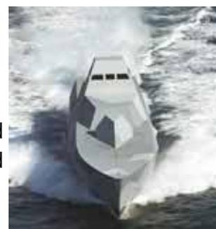
A stealth corvette of the YS 2000 design has a detection range of 13km in rough seas and 22km in calm sea without jamming. In a jammed environment, the Visby would be detected at a range of 8km in rough sea and 11km in calm sea.
